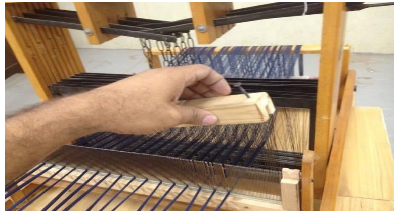
Form (9) the method of operation, opening of the reed and the change of denting during the weaving process.
